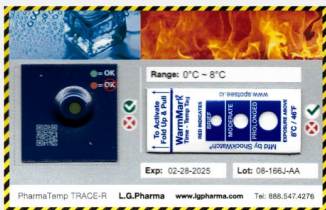
FIGURE 1 Temperature monitoring card is used while the product is in transit. Not to be used to monitor in-clinic refrigeration.
